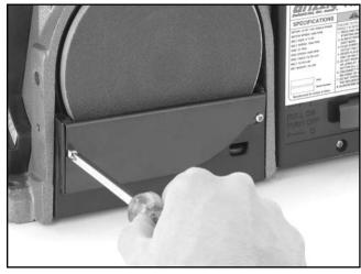
**Figure 4.** Attaching the disc guard.
